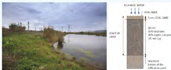
Figure 1: Left panel: An infiltration pond at Sant Vicenç dels Horts; right panel: schematic cross-section of the reactive organic layer
