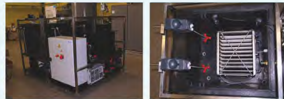
Figure 1: Pilot hybrid ceramic membrane filtration at a Swiss WWTP (left panel) with view from above on suspended ceramic membranes and agitators (right panel)
